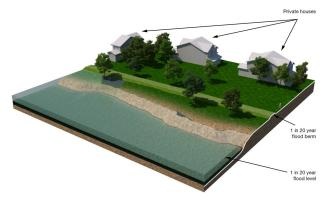
Figure 27 - Dyke Barrier
