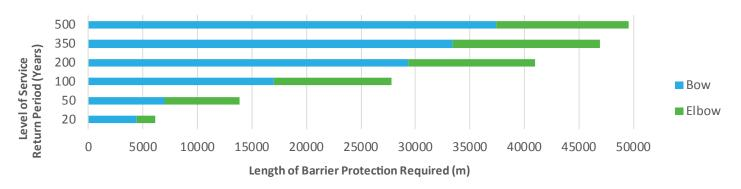
Figure 21 - Length of Barriers Required to Provide Various Levels of Service
