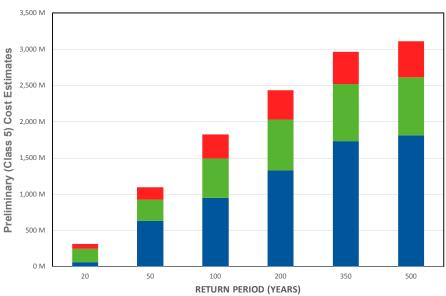
■Sum of Overland Cost ■Sum of Stormwater Cost ■Sum of Groundwater Cost Figure 19 - Cost of City Wide Flood Protection vs Return Period
