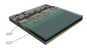
Figure 25 - Concrete Wall on Existing Barrier
