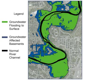
Figure 5 - Groundwater Inundation Mapping Example
