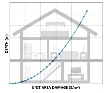
Figure 9 - Example Depth Damage Curve
