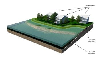
Figure 28 - Dyke Barrier
