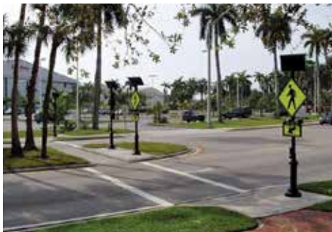
Figure 3.2-7: Rectangular rapid flash beacon
