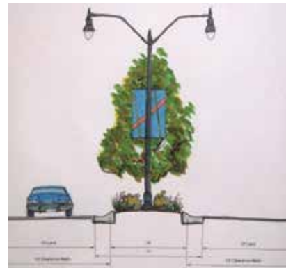
Figure 3.1-9: Street where turn lanes would not be appropriate
