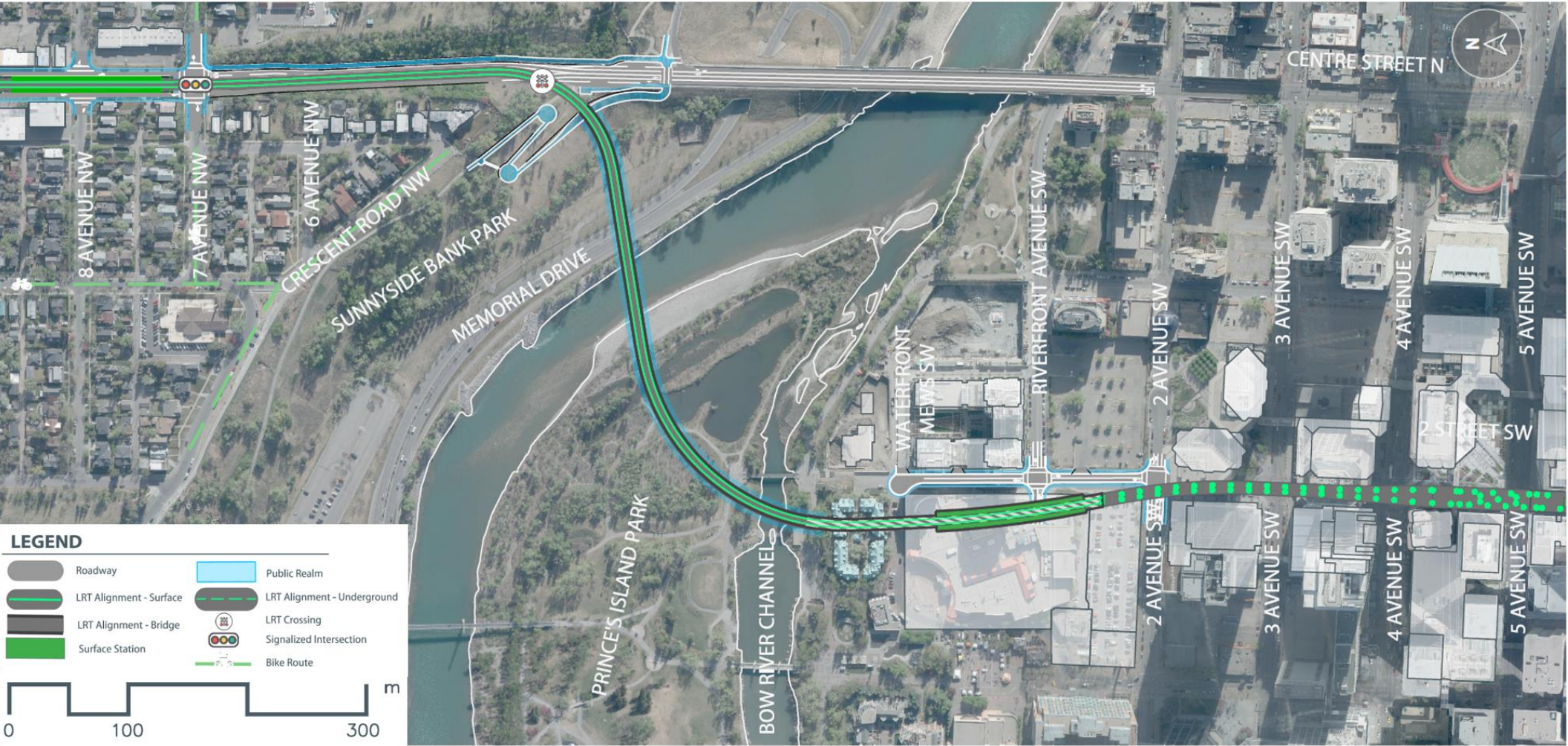
Figure 11. Bow River LRT Bridge alignment
