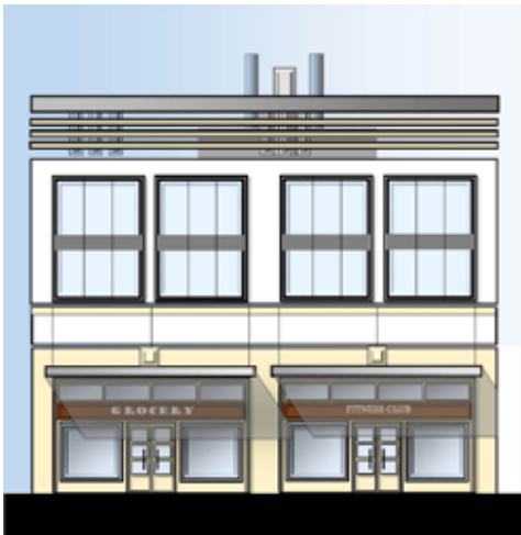
Partial or full screening of rooftop antennas minimizes visibility from a distance and from street level.
