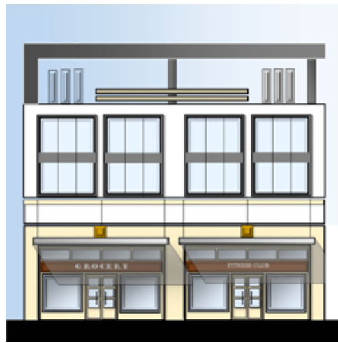
Partial or full screening of rooftop antennas minimizes visibility from a distance and from street level.
