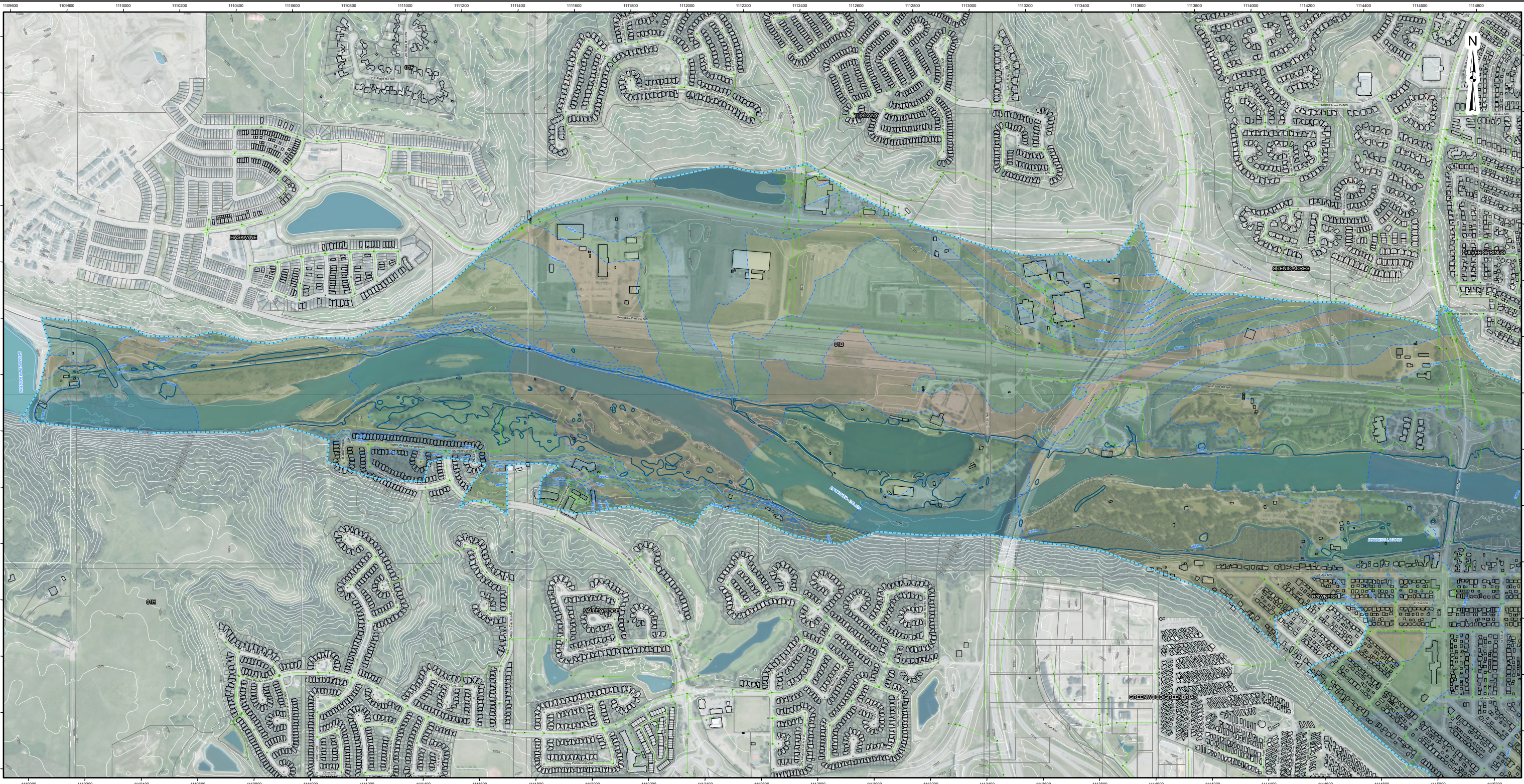
FIGURE 2.2 GROUNDWATER ELEVATION REPRESENTATION (P90) ANNUAL HIGH RIVER FLOW 1 - VALLEY RIDGE
