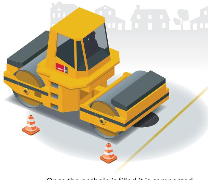
**4** Once the pothole is filled it is compacted using a roller. The asphalt is compacted until it is level with the roadway.
