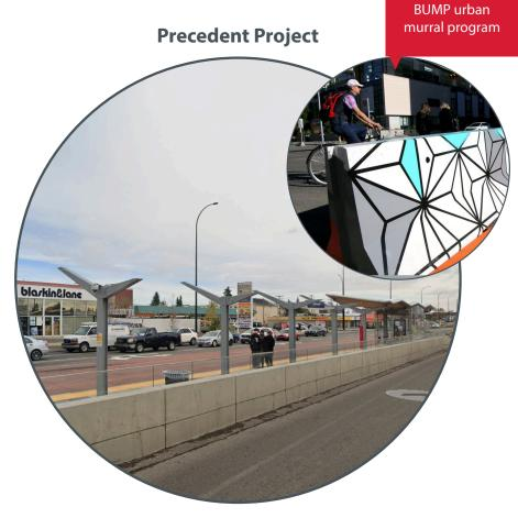
Example of a vertical concrete retaining wall on 17 AV SE in Calgary, Alberta. The vertical wall utilizes a smaller footprint in comparison to the jersey barrier and as a result provides more space to the pedestrian. The smaller image highlights a recent initiative by the Beltline Urban Mural Project (BUMP) to bring art to road infrastructure.
