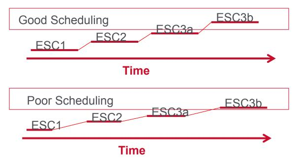
To prevent poor scheduling and reduce the risk of sediment loss during construction, the ESC Plan should take into account these transition periods. Use the drawing codes from the Construction Drawings section, including sub drawings (e.g. ESC2a, ESC2b), to populate the Transition Planning section. For instance, if you have the following drawings for a multi-family
